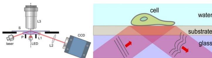
Fig. 4 THM interferometer setup and a detail of the THM prism configuration
