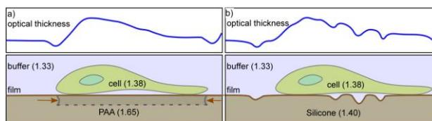
Fig. 2: Schematic of the cell-substrate sample (lower: a) PAA, b) silicone) and the corresponding optical thickness profiles (upper). The cell-silicone sample was taken from Ref [4] as the comparison.
